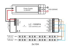
2)Receiver Connection Diagram for Multiple Units
