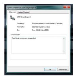
After the installation process is finished successfully you can find the entry under the node HID (Human Interface Devices) in the device manager.
