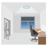
After hold-time, the light dims to stand-by level or switch off if the stand-by period is pre-set to Os.
