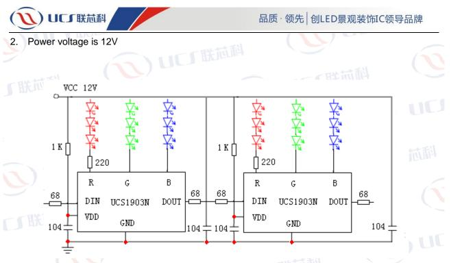
In order to prevent the damage of charged pull plug, when 12 v power supply, Din and Do all the string in a 68-80 ohm resistor for protection
