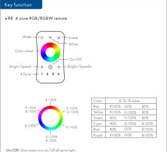
1,2,3,4 zone: Short press select and turn on zone light, long press 2s turn off zone light. Short press multiple zone key fastly, will synchronous select multiple zone synchronously.
