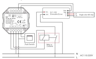
Note: We recommend the number of LED drivers connected to 0/1-10V dimmer does not exceed 5 pieces, The maximum length of the wires from dimmer to LED driver should be no more than 1.5 meters.
