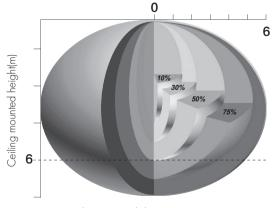
Ceiling mounted detection pattern (m)
