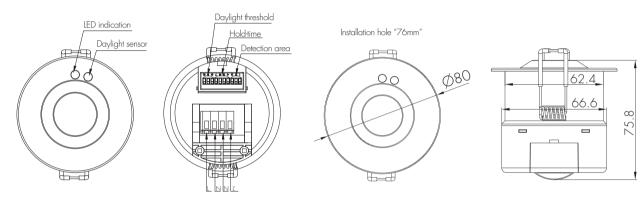
Note:We recommend the mounting distance between sensor to sensor should be more than 2m to prevent sensors from false-triggering.
