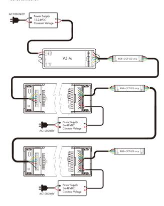
NOTE: The PWM input can be 5-24V or 36-48V, please select correct V+ wire terminal.
