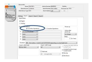
When using crossline operations for the destination address either a zone or a multiple line address (broadcast, group or shortaddress) can be selected:
