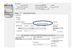
DALI-Line crossfunctions are supported for DALI MC+, DALI Switch, DALI MC4L, wDALI MC, wDALI Switch and wDALI Remote.
