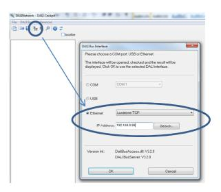
After IP-address is entered press "OK" to connect.
